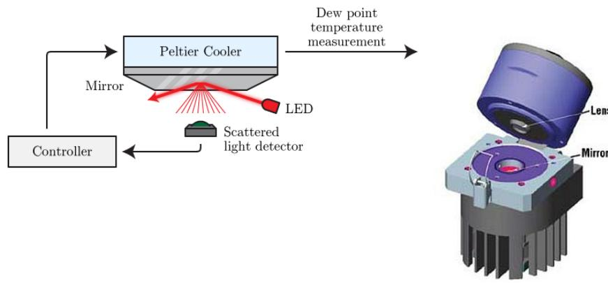
Condensation Hygrometers measure the Dew Point directly
