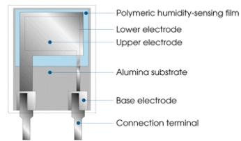
Another type are Electrical Hygrometers, also measuring Relative Humidity
