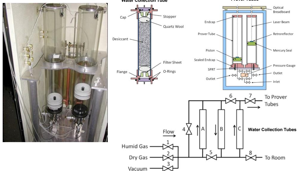
Gravimetric Hygrometers are the most accurate primary standards, measuring Specific Humidity
